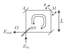
Now the mirror at A is tilted very slightly upwards, out of the plane of the experiment, by a small angle  $\psi$ . The tilt is too small to affect the overlap of the beams at BS, but it introduces a small phase  $2\phi$  between the clockwise and anti-clockwise paths, so that some light emerges at the output O.
