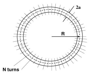
A toroid has a mean radius R and an inner radius a. It has N turns of thin wire wrapped uniformly around the toroid as shown in the figure, carrying a current I. Find an expression for the magnetic flux density in the toroid and hence determine the self-inductance of the circuit. For such a toroid with N=1000, R=1 m, a=5 mm, and I=20 A, evaluate the energy stored in the magnetic field.
